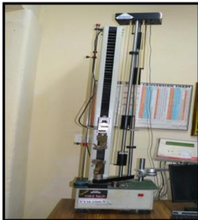
Figures; 1 Shear bond strength testing using universal testing machine
